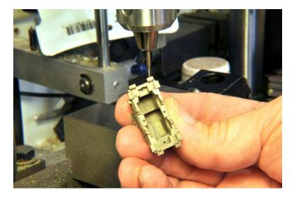
4. Chassis with all four holes drilled through.
