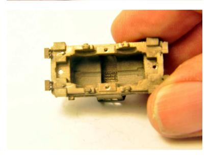
Completed chassis prep with all holes drilled, tapped, and cleaned up; wash chassis afterwards inside and out to remove any metal shavings which might later cause electrical shorts.
