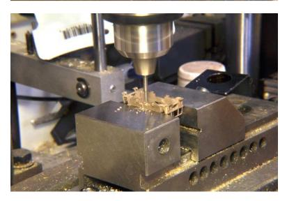
3. Drill holes at dimple locations (4) with #65 or 1mm drill. Hole should be all the way through at each location.
