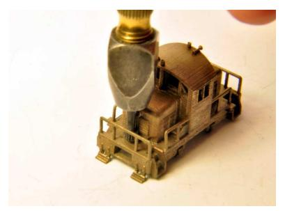
7. I remove the burr with a small metal countersinking tool.
