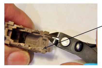
Using flush cutters, remove sprue to back of steps. No need to file or grind flush as the leftover nubs will not be visible.
