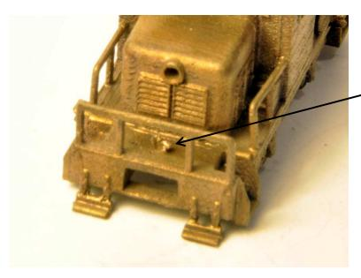
6. Drilling and tapping leaves burrs on the edges of the holes as shown here which must be removed.
