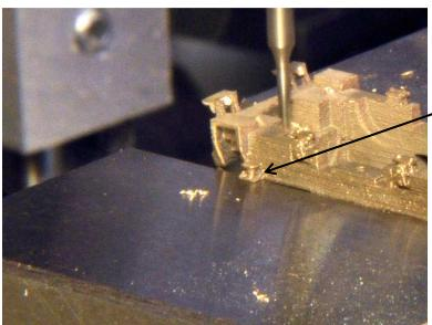
2. Clamp body casting in milling vise with bell brackets on both sides resting on top of vise.
