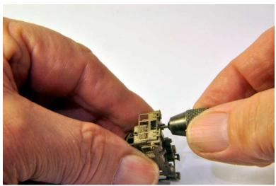
5. Tap holes with 00-90 tap. You can use one of the fancy tapping fixtures from Micro Mark, but I have not found it necessary, and just hand-tap as shown.
