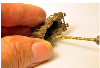
8. Alternatively, the burrs can be removed with a #40 drill bit, or with a file (taking care not to file off any of the detail on the top of the end platforms.
