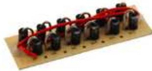
MRC AT880 Universal Voltage Reducer (AC/DC/DCC)
